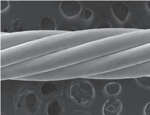
Image from a scanning electron microscope (200x magnification) of the surface quality of NiTi Ortho-Kabel 7 Twist™ with round cross-section.
